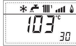
29. Visualisation solar probe temperature value S2 with solar board INSOL
