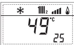
24. Visualisation safety thermostat with board ZONA MIX 2 (input S1) respectively ON and OFF
